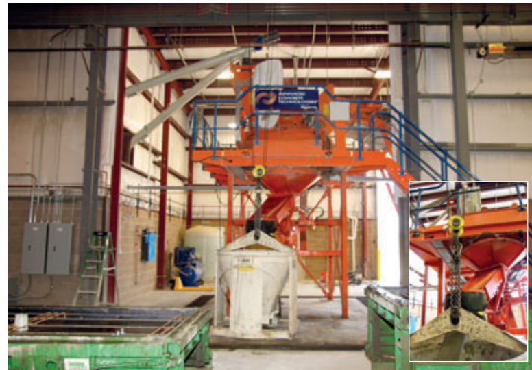
Fig. 3: Fully automated SmartMix 1125 batch plant with high shear Wiggert planetary HPGM 1125 mixer provides one cubic yard of output every 2.5 minutes. Two-position hydraulic swing chute provides flexible filling options. White crane bucket in front of mixer and green trench forms in foreground.
