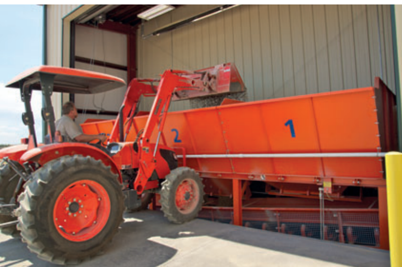
Fig. 4: Lee Wheeler, Trenwa plant production manager uses a front end loader to charge aggregate bins outside the recently upgraded Colorado plant. The bins store crushed stone, sand and pea gravel for a total of 44 tons capacity.
